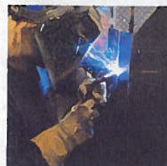
Rock Auger running a vertical bead with a MIG welder.
