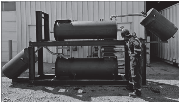
The five-tonne Endpoint Recovery waste disposal unit, which turns organic garbage into diesel, graphite and water.
